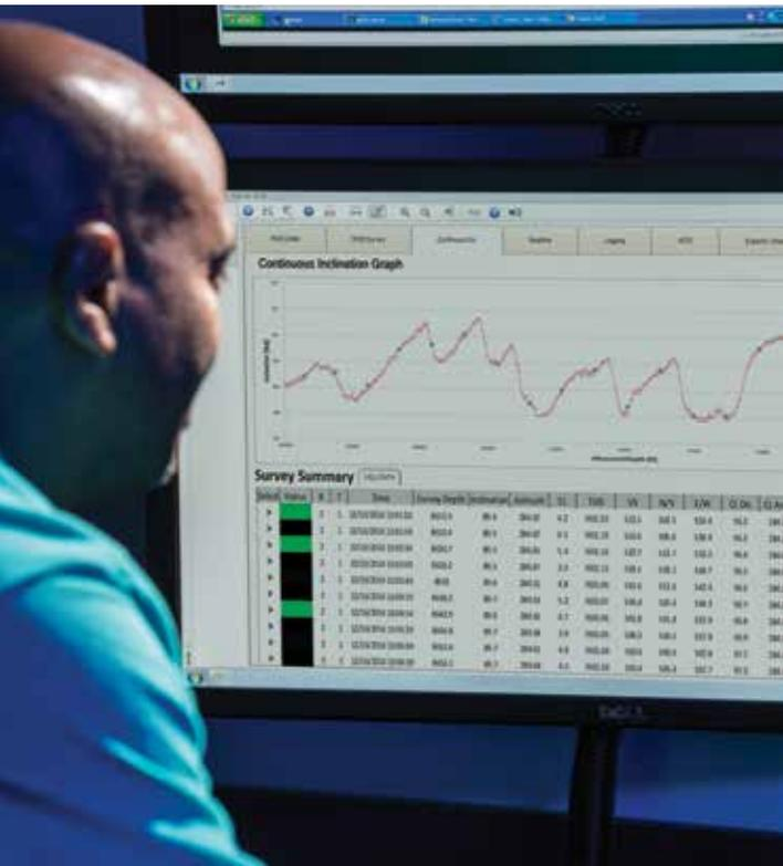
*The continuous inclination measurements offers greater resolution to optimize wellbore placement.*
